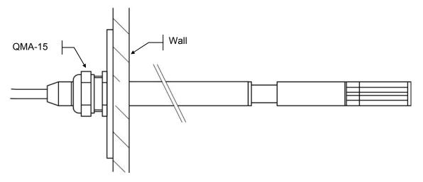
Installation Note: You may want to provide an orifice at a distance of about 3" from the probe of the transmitter for future use by a reference probe and HygroPalm indicator.
